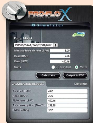
Operators can use Wilden's free PX Simulator (on [www.wildenpump.com/seemoregreen](http://www.wildenpump.com/seemoregreen)) to see how adjusting the dial on their Pro-Flo X™ ADS can improve the efficiency of their pumps.
