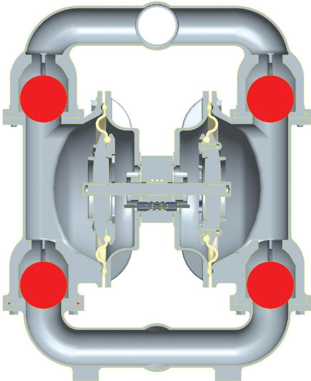
A cross section of the Wilden® Advanced™ Series 3-inch stainless steel “drop-in” wetted path. It features a larger cross sectional area (compared to a traditional 3-inch stainless-steel wetted path) to reduce internal friction losses.
