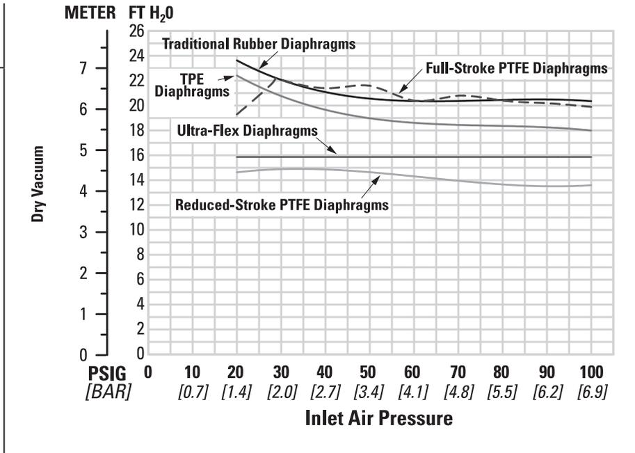
Suction-lift curves are calibrated for pumps operating at 305 m (1,000') above sea level. This chart is meant to be a guide only. There are many variables that can affect your pump's operating characteristics.
