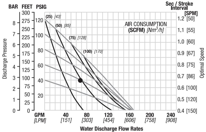
Flow curves are for "optimal speed" conditions only. The "optimal speed" is that speed which provides the maximum flow under a particular air and fluid pressure condition. The optimal speed varies for different fluid and air pressures. Recommendations for optimal speed can be found on the right side of the flow curve.
