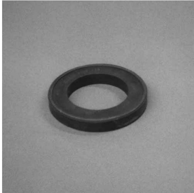
When reinstalling elastomeric valve seats, make sure the beveled surface mates with the manifold for proper sealing characteristics.
