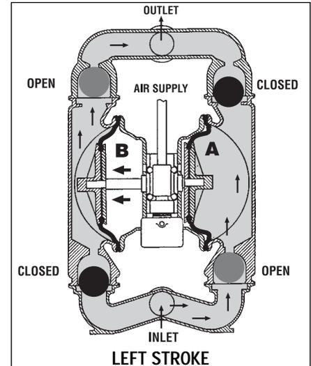
**FIGURE 3** At completion of the stroke, the air valve again redirects air to the back side of diaphragm A, which starts diaphragm B on its exhaust stroke. As the pump reaches its original starting point, each diaphragm has gone through one exhaust and one discharge stroke. This constitutes one complete pumping cycle. The pump may take several cycles to completely prime depending on the conditions of the application.
