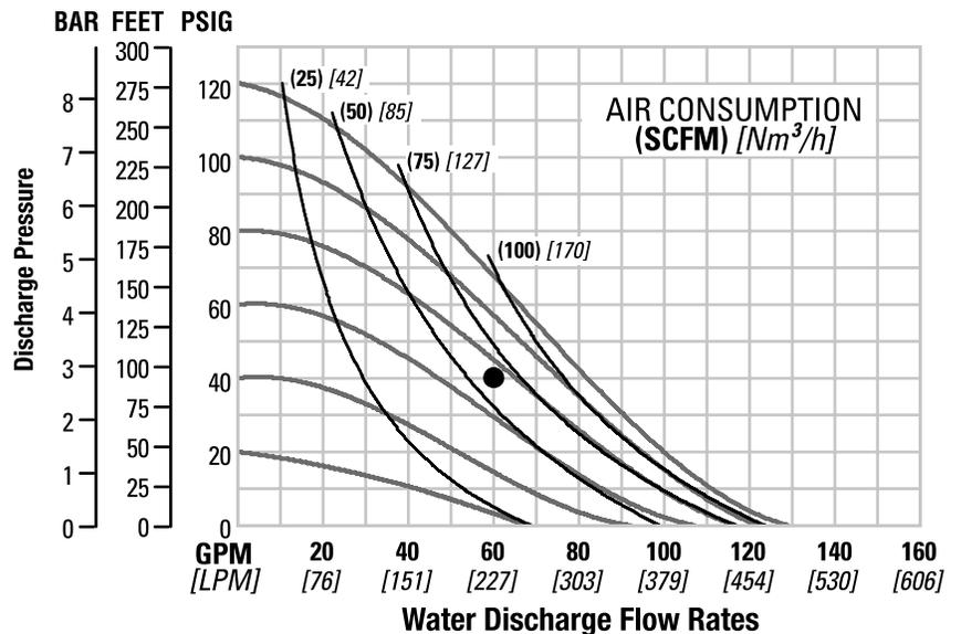
Flow rates indicated on chart were determined by pumping water with a vertically mounted, center ported ball check configuration. When alternate check valve options are used, multiply flow rate by appropriate factor. For optimum life and performance, pumps should be specified so that daily operation parameters will fall in the center of the pump curve.
