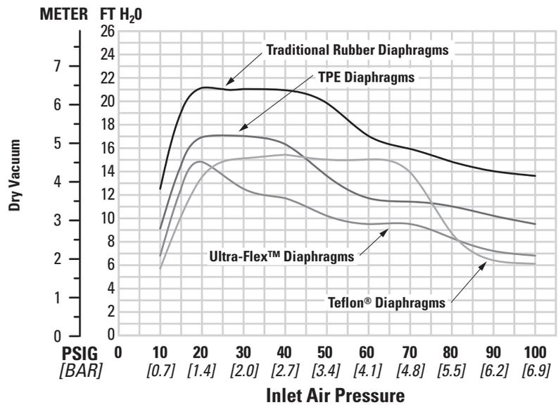
Suction lift curves are calibrated for pumps operating at 305 m (1,000') above sea level. This chart is meant to be a guide only. There are many variables which can affect your pump's operating characteristics. The
