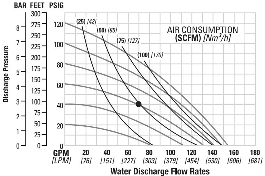
Flow rates indicated on chart were determined by pumping water with a vertically mounted, side ported ball check configuration. When alternate check valve options are used, multiply flow rate by appropriate factor. Mushroom check valve = 93%, flap check valve = 143%. For optimum life and performance, pumps should be specified so that daily operation parameters will fall in the center of the pump performance curve.
