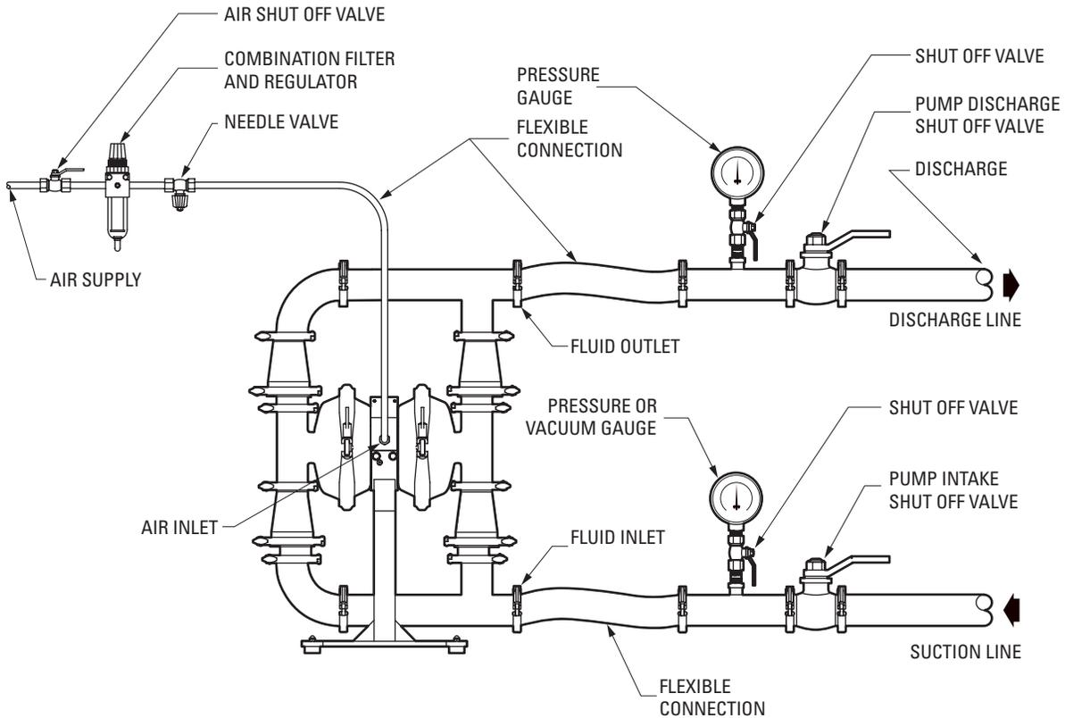
**NOTE:** In the event of a power failure, the shut off valve should be closed, if restarting of the pump is not desirable once power is regained.
