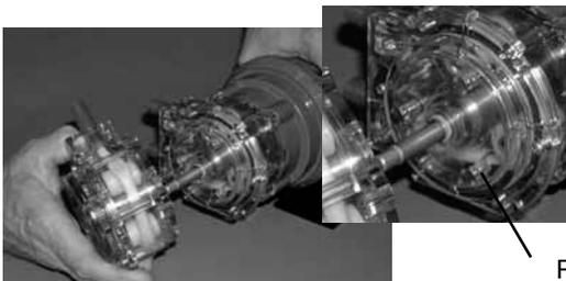
**Step 5.** When attaching the outside tube housing to the unit, align the three rivets of the inside tube housing with the matching rivet holes of the outside tube housing. Once in place, turn outside side tube housing counter-clockwise to lock it in place.
