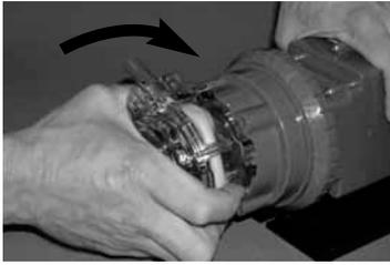
**Step 1.** Switch off the feeder and unplug the power cord. Hold the feed rate control section and turn the complete tube housing clockwise until it stops.
