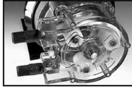
**CAUTION:** Pump fresh water through the tubing to clean out chemicals then let pump run dry for a couple of cycles. Use caution when disconnecting feed pump lines, changing the tube or the tube housing. They may contain hazardous chemicals. Protective eye gear, hand gear and clothing should be worn at all times during service to prevent chemical contact. For easier tube changing, reverse the feed pump in the wall mounting bracket so that pump housing is facing upward.
