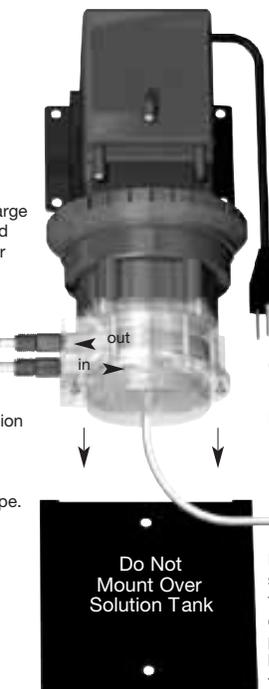
Insert a length of 1/4" suction/discharge tubing into the newly created hole and place the other end back into the solution tank.
