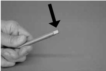
**Step 3.** When replacing the original shaft with the dual head shaft, be sure to insert the end with the flat surface first. (Figure 3) Once inserted, gently twist until shaft drops in place. (Figure 3A)
