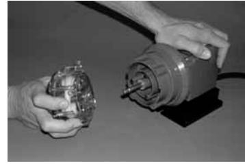
**Step 2.** Pull the complete tube housing straight out. Use pliers to remove main shaft from feed rate control section.
