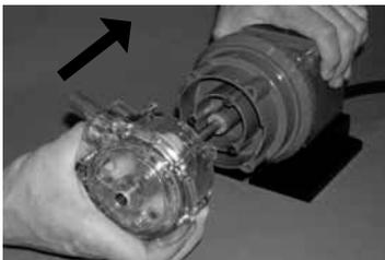
**Step 4.** Grease the tip of main shaft and insert the inside tube housing (three rivets are visible on the tube housing cover) then slide the shaft completely through. (Figure 4) Align the tube housing so that the inlet and discharge face the left side of the motor. Be sure to line up the three feed rate rivets on the pump motor unit with the matching rivet holes of the tube housing. (Figure 4A) Once in place, turn inside tube housing counter-clockwise to lock it in place.
