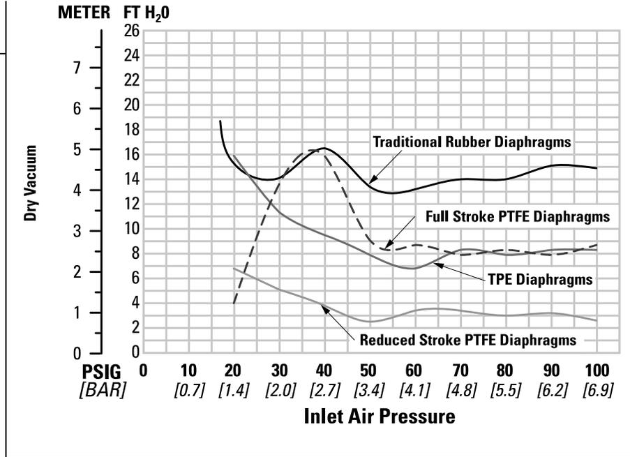
Suction lift curves are calibrated for pumps operating at 1,000' (305 m) above sea level. This chart is meant to be a guide only. There are many variables which can affect your pump's operating characteristics. The number of
