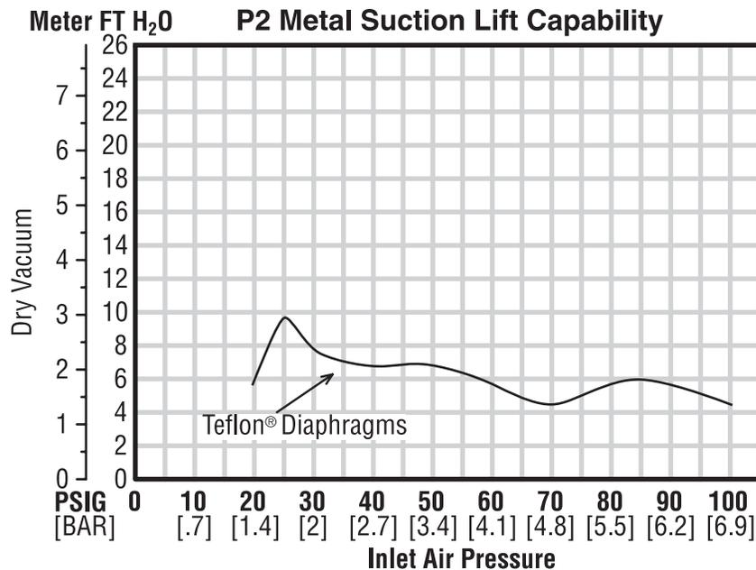
Suction lift curves are calibrated for pumps operating at 305 m (1,000') above sea level. This chart is meant to be a guide only. There are many variables which can affect your pump's operating characteristics. The number of intake and
