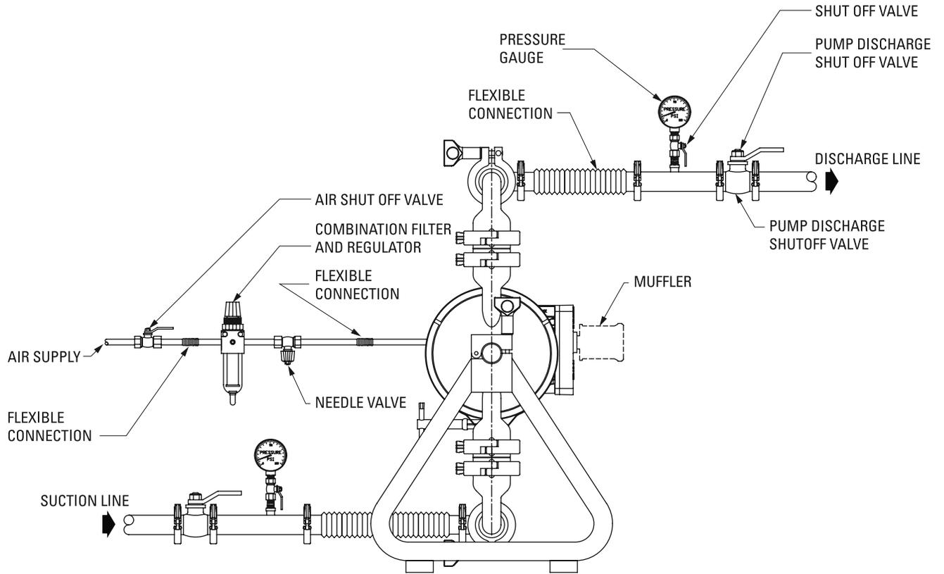
**NOTE:** In the event of a power failure, the shut off valve should be closed, if restarting of the pump is not desirable once power is regained.
