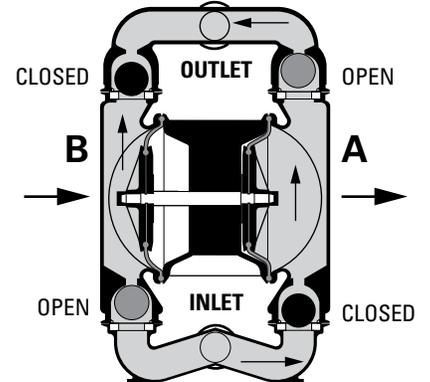
**FIGURE 3** At completion of the stroke, the air valve again redirects air to the back side of diaphragm A, which starts diaphragm B on its suction stroke. As the pump reaches its original starting point, each diaphragm has gone through one suction and one discharge stroke. This constitutes one complete pumping cycle. The pump may take several cycles to completely prime depending on the conditions of the application.
