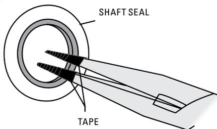
**SHAFT SEAL INSTALLATION:**
