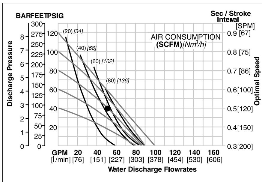
Flow curves are for “optimal speed” conditions only. The “optimal speed” is that speed which provides the maximum flow under a particular air and fluid pressure condition. The optimal speed varies for different fluid and air pressures. Recommendations for optimal speed can be found on the right side of the flow curve.
