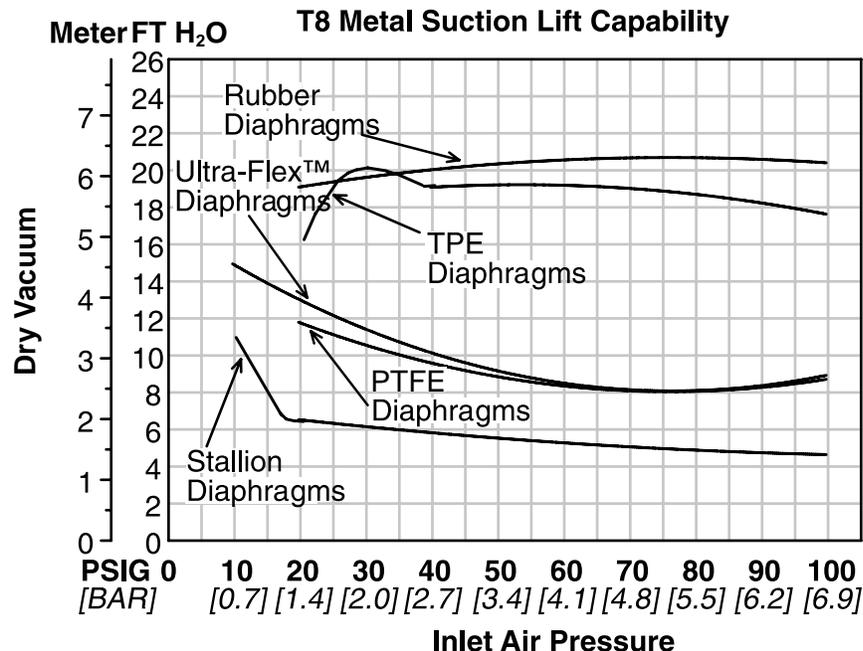
Suction lift curves are calibrated for pumps operating at 305 m (1,000') above sea level. This chart is meant to be a guide only. There are many variables which can affect your pump's operating characteristics. The number of intake
