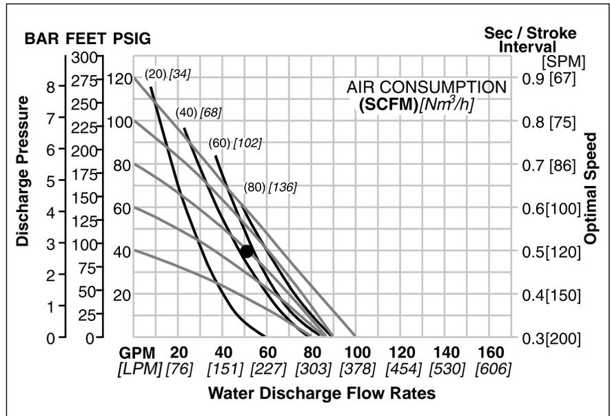
Flow curves are for "optimal speed" conditions only. The "optimal speed" is that speed which provides the maximum flow under a particular air and fluid pressure condition. The optimal speed varies for different fluid and air pressures. Recommendations for optimal speed can be found on the right side of the flow curve.
