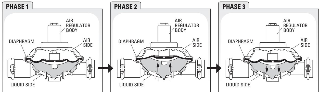
A compressed air line attached to the air regulator body sets and maintains pressure on the air side of the diaphragm. As the reciprocating pump begins its stroke, liquid discharge pressure increases which flexes the Equalizer® diaphragm inward. This action accumulates fluid in the liquid chamber (see Phase 2) and the air regulator allows compressed air to enter the air side. When the pump redirects its motion
