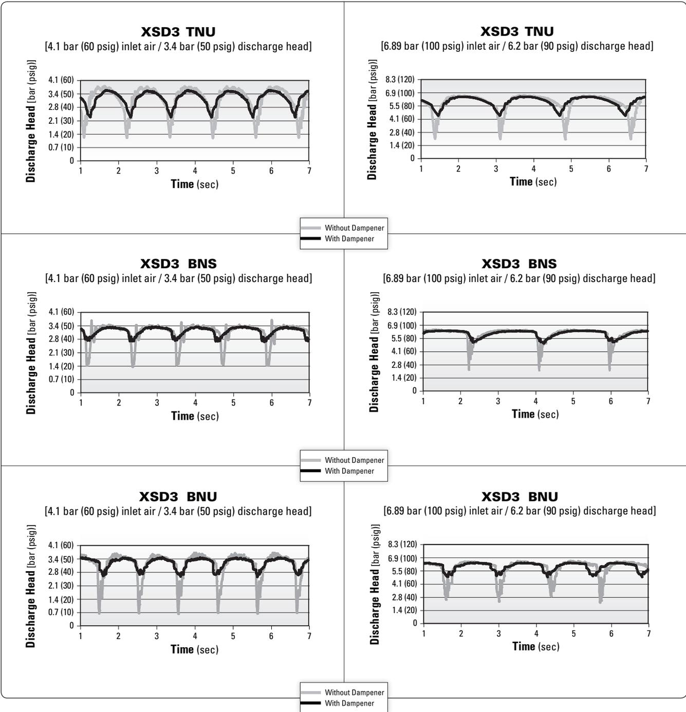
These charts show discharge head fluctuations for a diaphragm pump with and without a dampener. By reviewing the variation in pressure, the level of dampening can be estimated for an application. For example (XSD3 BNU 100/90), the head pressure generated by a 76 mm (3") pump operating at 6.89 bar (100 psig) air inlet pressure and 6.2 bar (90 psig) head pressure varies
