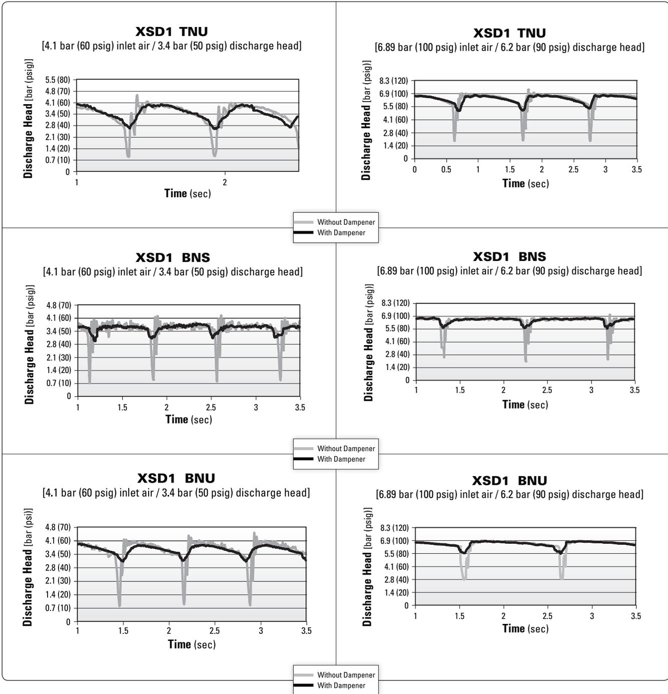
These charts show discharge head fluctuations for a diaphragm pump with and without a dampener. By reviewing the variation in pressure, the level of dampening can be estimated for an application. For example, the head pressure generated by a 25 mm (1") pump operating at 6.89 bar (100 psig) air inlet pressure and 6.2 bar (90 psig) head pressure varies between 1.7 bar (25 psig) and 7.2
