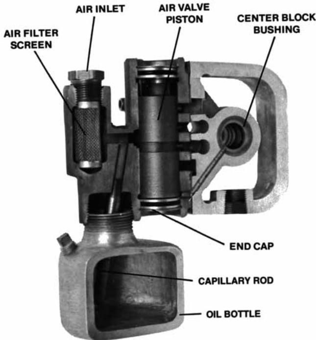
The air valve assembly consists of both the air valve body and piston and the center block. The unique design of the air valve relies on differential pressure to effect the diaphragm shift. It is reliable and simple to maintain. The bushing in the center block, along with the diaphragm shaft, provides the “trigger” to tell the air valve to shift. The following procedure will ensure that the air valve on your Wilden pump will provide long-lasting trouble-free service.
