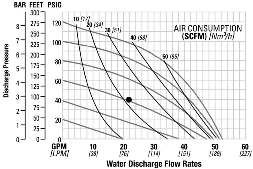
**Example:** To pump 83.3 lpm (22 gpm) against a discharge head of 2.8 bar (40 psig) requires 4.1 bar (60 psig) and 36 Nm³/h (23 scfm) air consumption.
