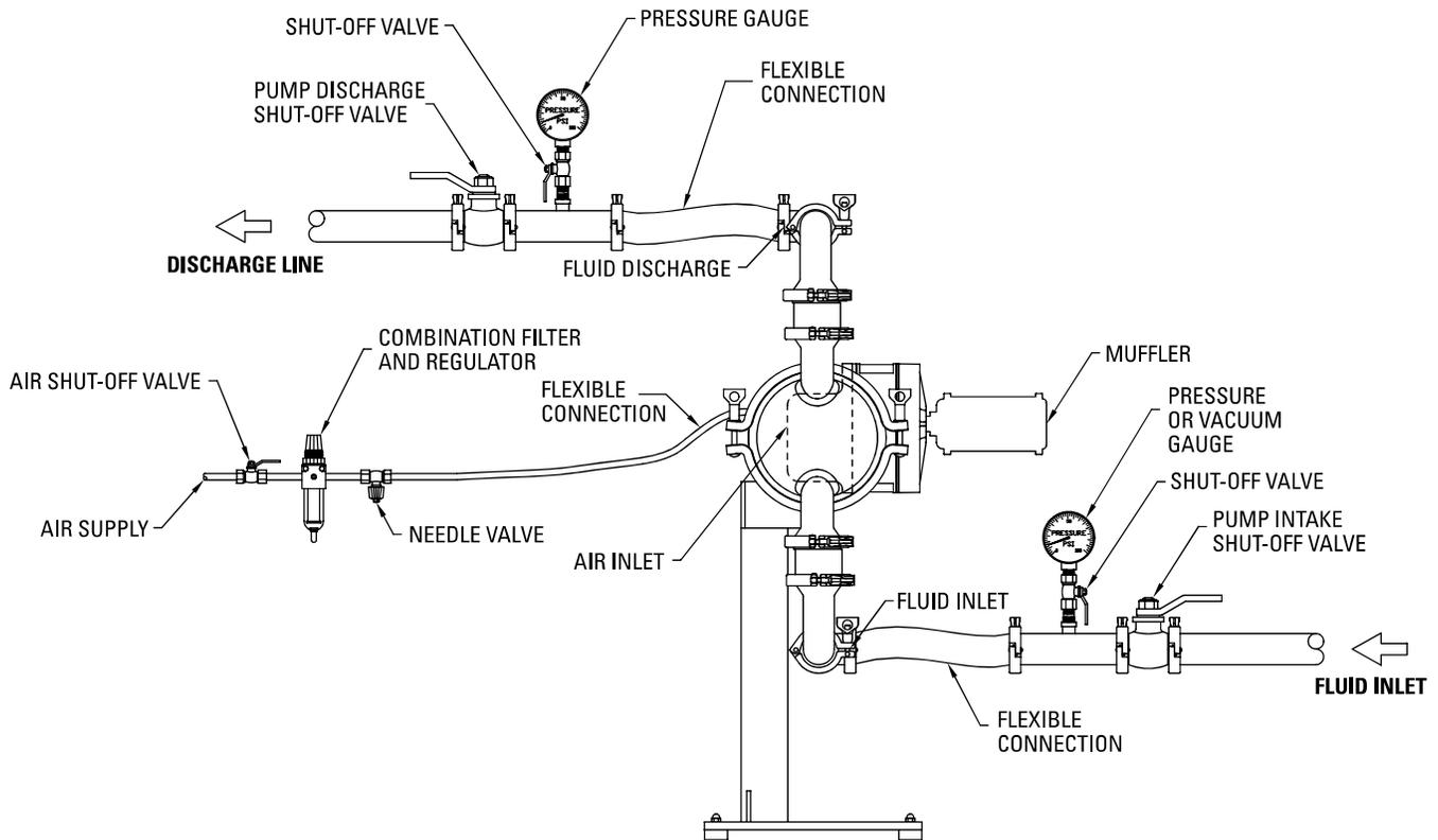
**!** **NOTE:** In the event of a power failure, close the shut-off valve if you do not want the pump to restart when the power returns.
