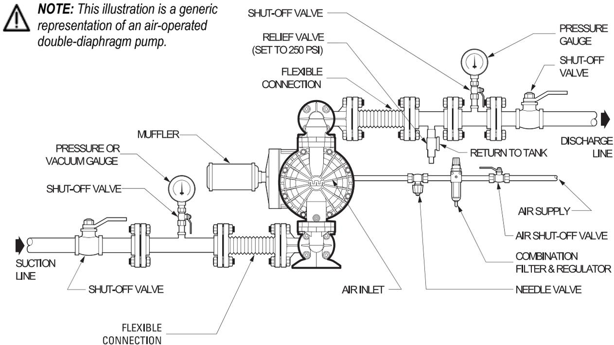
**⚠ NOTE:** In the event of a power failure, the shut-off valve should be closed, if restarting of the pump is not desirable once power is regained.
