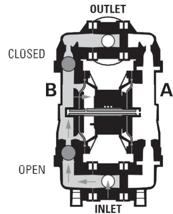
**FIGURE 3** At completion of the stroke, the air valve again redirects air to the back side of the diaphragm A, which starts diaphragm B on its exhaust stroke. As the pump reaches its original starting point, each diaphragm has gone through one exhaust and one discharge stroke. This constitutes one complete pumping cycle. The pump may take several cycles to completely prime depending on the condition of the application.
