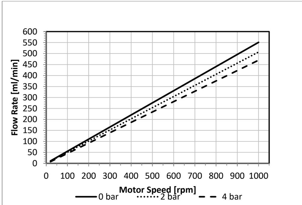
The flow rates showing at the chart above were ascertained with a new pump chamber under standard conditions after the final assembly of the pump.
