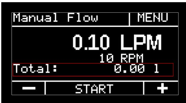
Picture 32 Manual Flow; totalizer (example)
