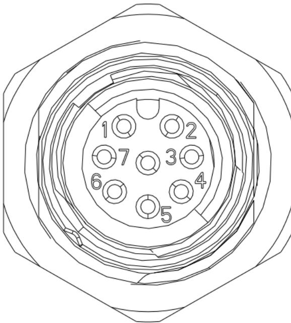
*Figure 1 Connection jack and pin-allocation*
