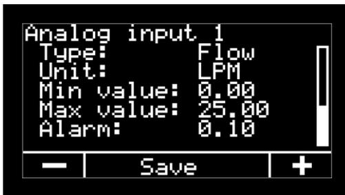
Picture 15 Analog input; configuration, part 2 (example)
