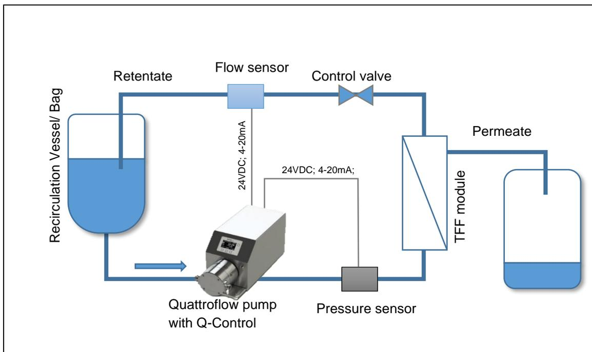
Picture 54 Example of setup for tangential flow filtration (TFF)
