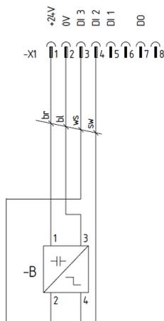
Picture 2 Connection example, Diaphragm monitoring, Port X1
