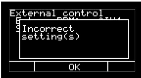
Picture 33 Error message; External control; Incorrect settings
