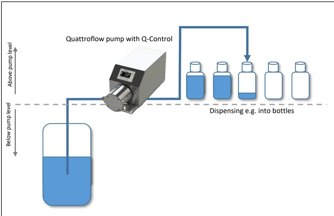
Picture 41 Example of a setup for a filling application
