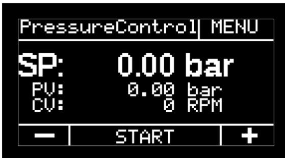
Picture 44 Pressure-Control; main window (example)
