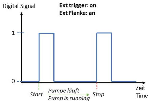
Picture 77 External Start/Stop, Ext. trigger ON, digital
