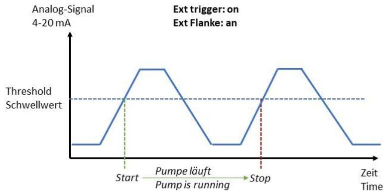
Picture 76 External Start/Stop, Ext. trigger ON, analog
