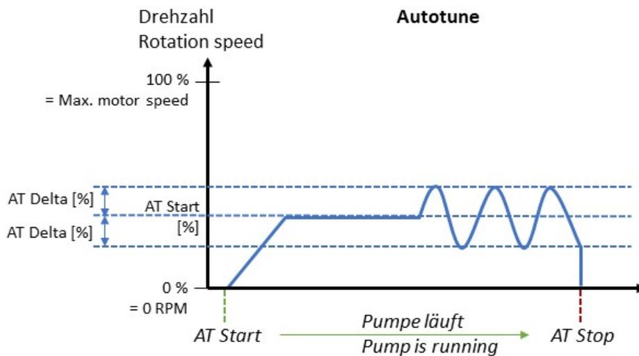
Picture 46 Flow- and pressure control; exemplary progress of the autotune
