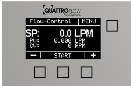
**Operator and Control Unit for Quattroflow pumps
