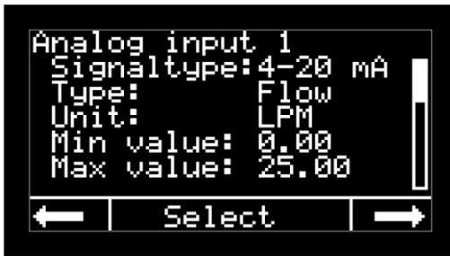
Picture 14 Analog input; configuration, part 1 (example)
