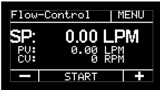
Picture 43 Flow-Control; main window (example)
