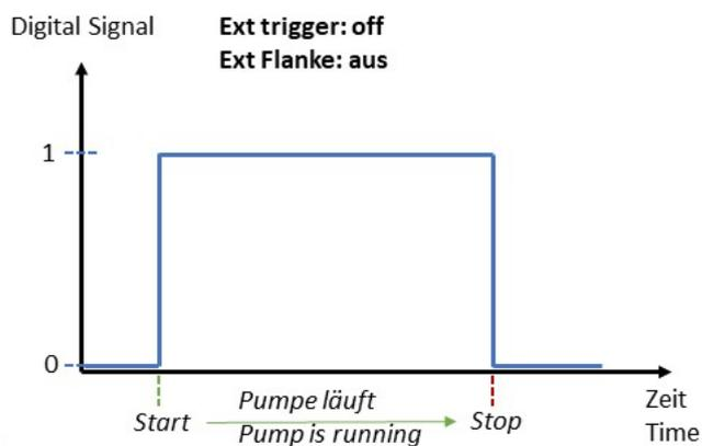
Picture 75 External Start/Stop, Ext. trigger OFF, digital
