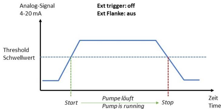
Picture 74 External Start/Stop, Ext. trigger OFF, analog
