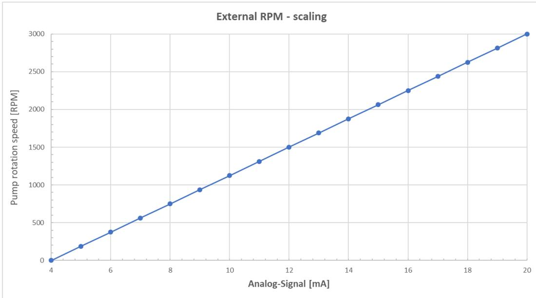
Picture 35 Graph for scaling current signal for mode External RPM; example for QF150QCon (max. 3000 RPM)
