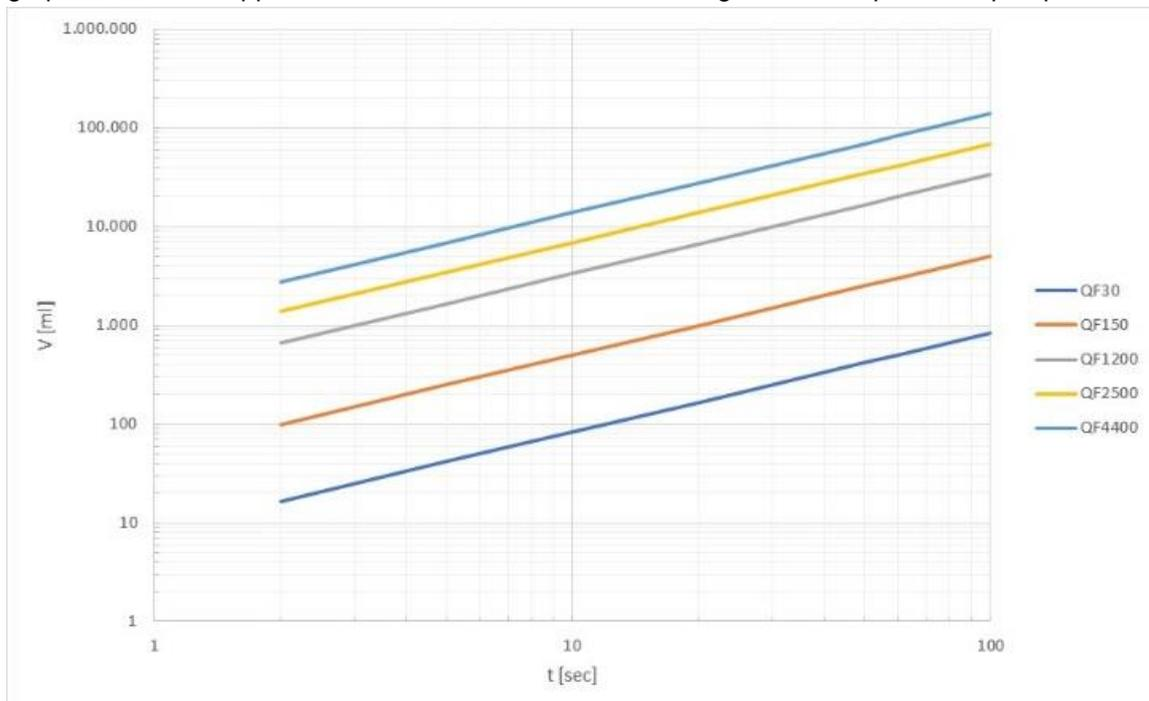
Picture 42 Maximum filling volume per unit of time
