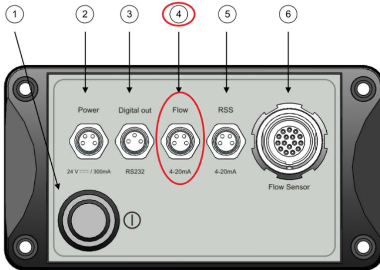
Figure 16: Rear view of BioProTT™ FlowTrack
