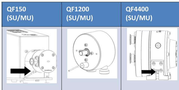
Picture 25 Quattroflow diaphragm monitoring; Example for installation
