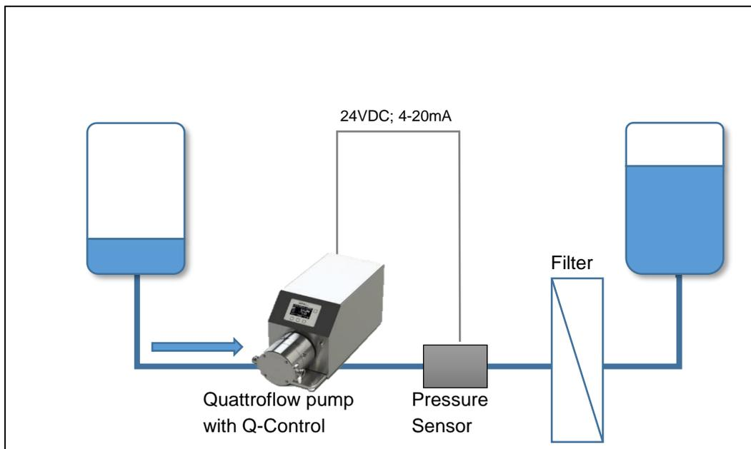
Picture 53 Example of a filtration setup with pressure control
