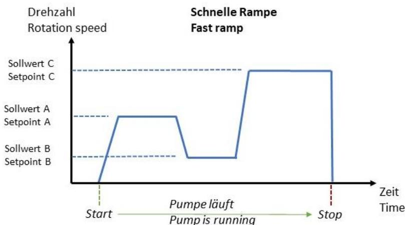
Picture 70 Example for a fast slope
