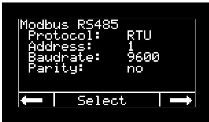
Picture 89 RS485 Modbus configuration
