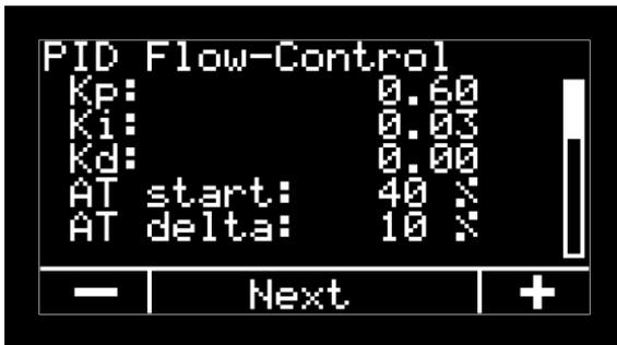
Picture 45 Flow-Control; configuration (example)
