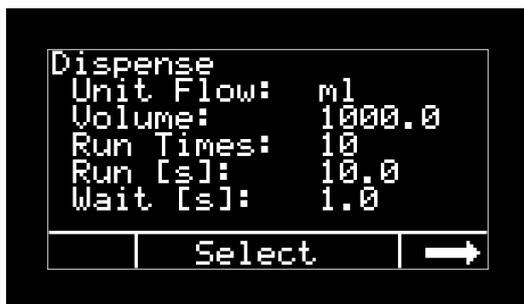
Picture 39 Parameter settings for filling mode
