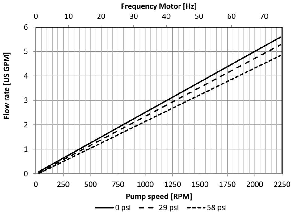
The flow rates showing at the charts above were ascertained with new diaphragms and new valves under standard conditions after the final assembly of the pump. Depending on the selected motor/frequency drive combination, the motor frequency and the resulting pump speed might differ.
