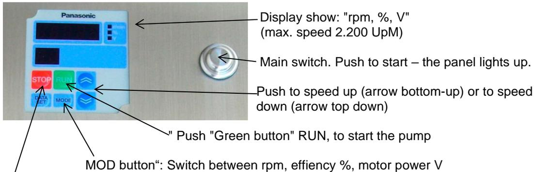
Push the "Red button" STOP to stop the pump
