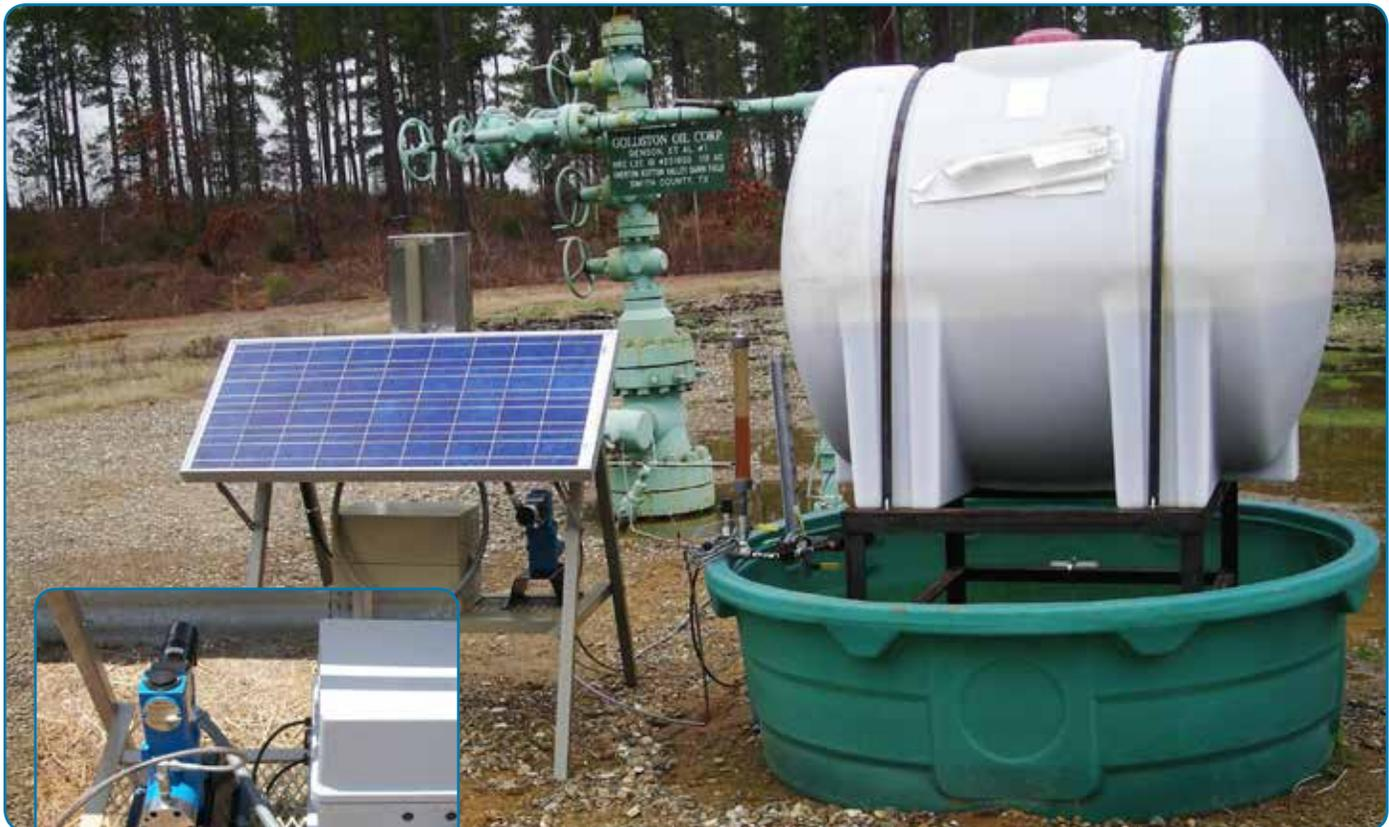
Neptune™ Solar D™ Chemical Injection Pumps have proven to be an accurate, consistent, durable and reliable way to inject corrosion inhibitors into a well bore, while their being solar-powered reduces the need for on-site maintenance and costly trips to the well site by oilfield technicians.
