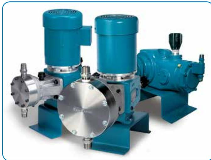
Neptune™ 7000 Series Mechanical Diaphragm Metering Pumps are ideal for dosing alum and ferric chloride because they do not feature contour plates on the liquid side of the diaphragm, resulting in a simple, straight-through valve and head design that allows improved flow characteristics.
