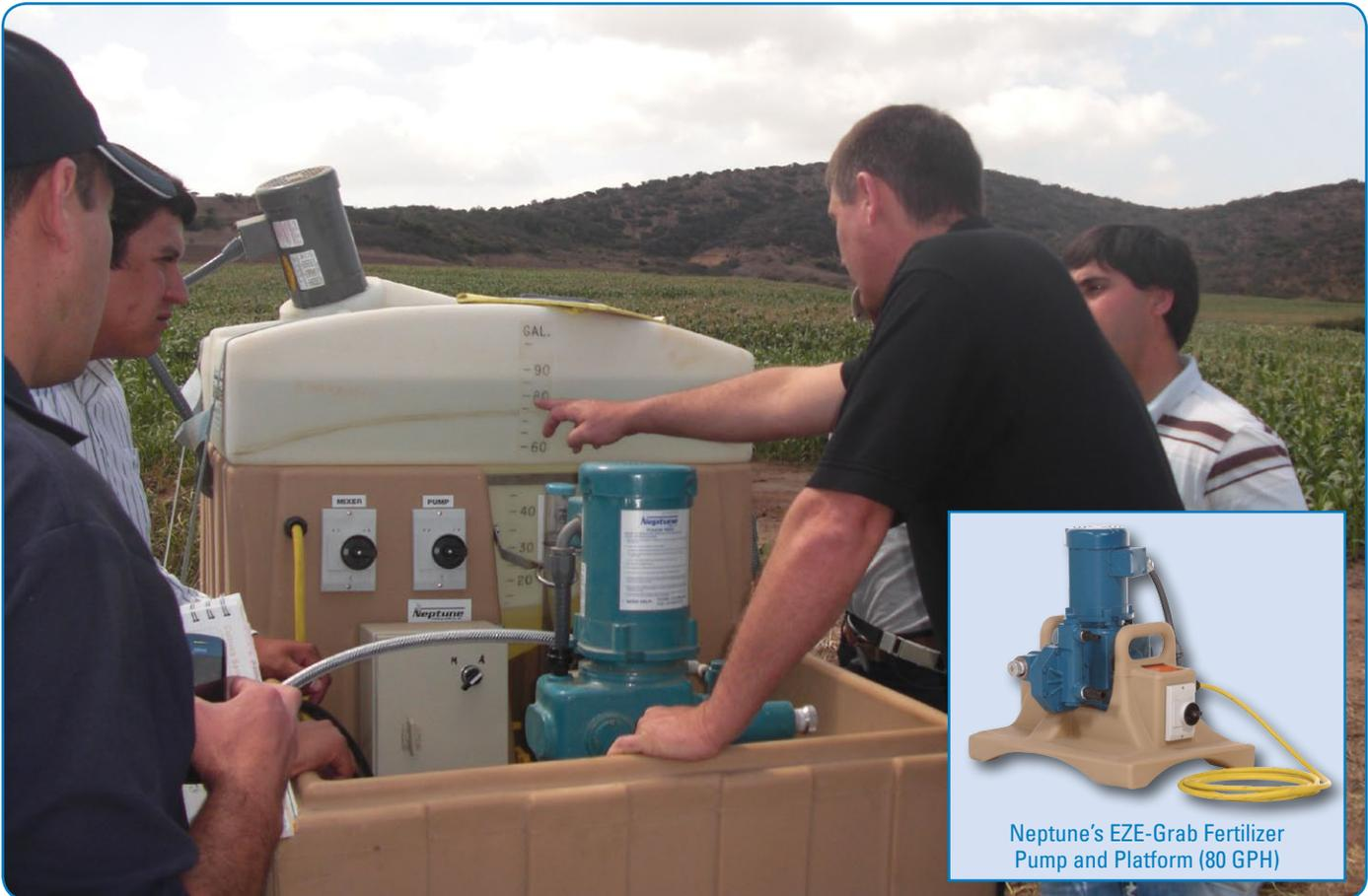
A chemigation system featuring a Neptune Series 500 metering pump is perfect for use with a center-pivot watering system due to the pump's ability to deliver precise amounts of fertilizers and chemicals at the precise time.
