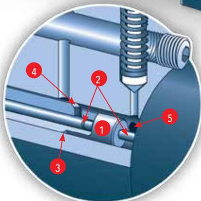
Turning the micrometer dial moves the metering rod and changes the pump capacity. When the metering rod is moved in, the tip of the metering rod closes port **4** sooner in the stroke allowing for less by-pass and more pumping action. Likewise, when the metering rod is moved out, the tip of the metering rod closes port **4** later in the stroke allowing more by-pass and less pumping.
