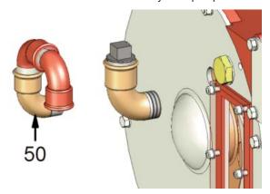
Assemble complete vacuum kit on pump cover.
