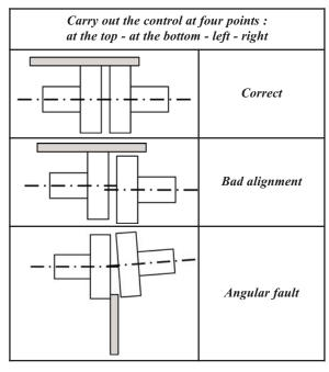
It is important to control the alignment at every step of installation in order to ensure that none of these steps generates stress on the pump unit or the pump itself:
