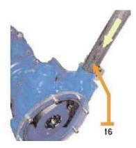
Insert the loose end of the hose **16** in the inlet port of the pump body **1**.
