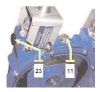
Fill the pump body with lubricant (see § LUBRICATION). Tighten plugs 11 and 23 in the body.
