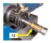
Fit bracket 18 on insert 12 and screw it on the body using screws 48 and washers 49.
