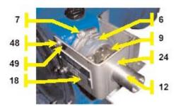
Fit snap ring **24** in the groove provided for this purpose on the insert.
