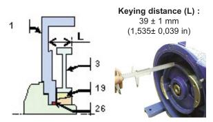
After checking that the expansible hub is properly centered with regard to the wheel thickness, gradually tighten screws **19a** while keeping wheel alignment correct.
