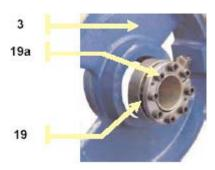
Remove the wheel 3 by sliding it along the central axis.
