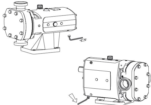
**Step 7****Removing seal retainers**
