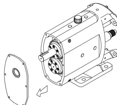
**Step 9****Removing timing gears**
