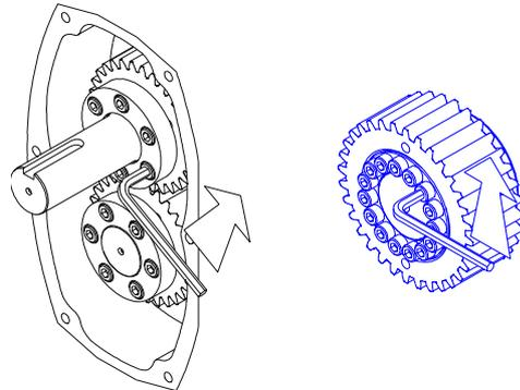
**Step 10****Shaft assembly removal**
