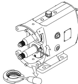
**Step 8****Removing Gearcase Cover**
