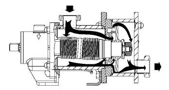
• A centrifuge pump is used for CIP cycles. This pump is placed upstream of the C Series pump.
