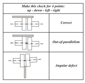
Controlling the alignment at each stage of the installation is important to be sure that none of these stages have generated stresses on the unit or the pump:
