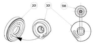
Place thread locking adhesive (Loctite® 243\* or equivalent) on the thread of the transmission hub 596.  Hold the piston 301 with a 46 Open-end spanner or a monkey wrench and screw-up the nut 304 after mounting the seal 305 on to the rear face.
