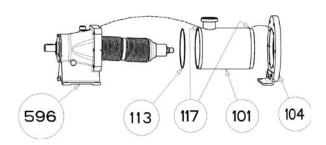
Assembly is undertaken in the reverse order of dismantling, taking care to correctly position the seal 113 and the 2 indexing pins 117. The nuts 115 must be re-mounted with thread locking adhesive (Loctite® 243\* or equivalent):
