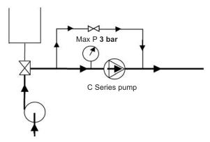
It is preferable not to run the C Series pump during CIP, although low speed (< 100 rpm) is acceptable by alternating start/stop operation.
