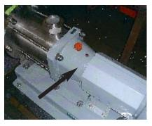
Verification of the correct rotation direction : Turn the pump the wrong way is not dangerous for the pump.
