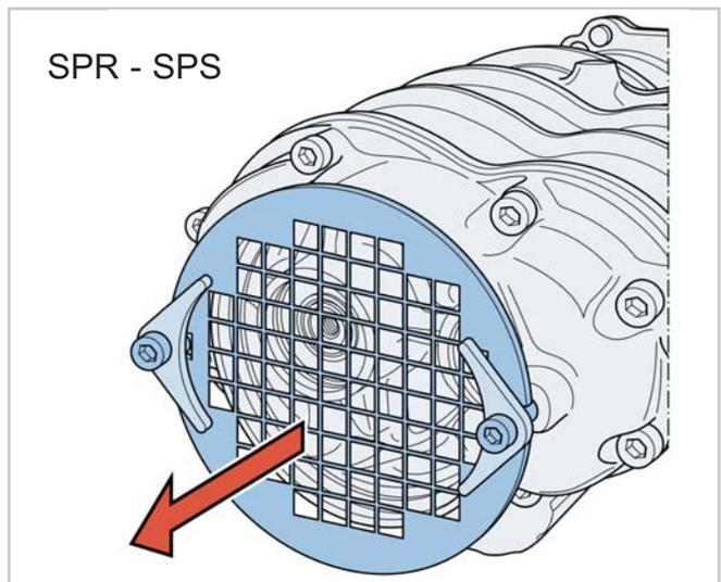
After speed regulation, remove the protection grid.
