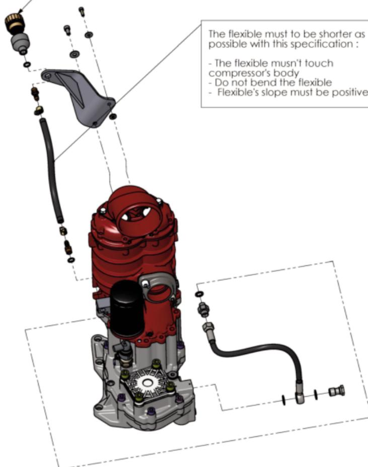
The flexible must to be shorter as possible with this specification :
