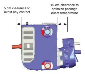
In the same way, a minimum distance of 5 cm must be respected between all accessories located in the chassis (PTO, universal joint, ...) and the compressor package.
