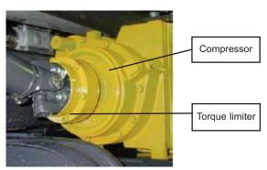
DDIC packages may be ordered with torque limiters mounted. Refer to Instructions 1401-B00 TORQUE LIMITER - MISTRAL B600 TYPHON II.
