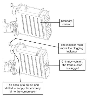
If this is the case, the air must be fed to the compressor from the rear of the filter box, on the boss, of diameter 140cm for the purpose.
