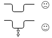
If installation is heated, it must be designed so that fluid dilatation can evacuate through piping. Therefore fluid contained in piping must be heated before fluid contained in the pump. Also check that a heated pump is not isolated by closed valves.
