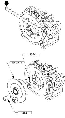
Lubricate the friction surfaces of the piston 12301O with a product compatible with the pumped liquid.
