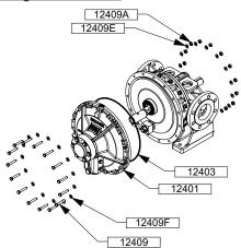
Remove the front cover bolts (screw 12409, nuts 12409A and washers 12409E - 12409F).
