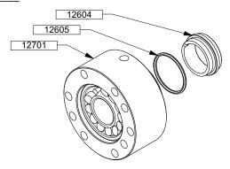
Remove the stationary seal face 12604 and its seal 12605.
