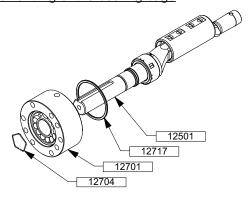
Remove the seal 12717 and check its condition. Replace it if necessary.
