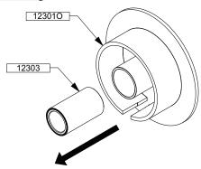
Remove the bushing 12303 of the piston 123010 with a press and a cylinder.
