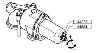
Setting is correct when flow rate is conform to expectation and when motor endures without incident absorbed power peak when discharge is closed. This is how relief valves of complete pumping sets are set, basing on information given to our technical services.
