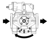
The reverse of the direction of rotation should be done after a full stop of the pump.
