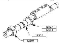
Check shaft 12501 surface condition. Rub it down with thin sand paper if there are scratches on seal rotating part O-ring place. In particular, it must be check that there are no scratches parallel to shaft axis.
