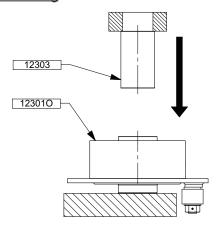
Insert the bushing 12303 in the piston 12301O with a press and a cylinder until the faces of the bushing and the piston are aligned (on both sides).
