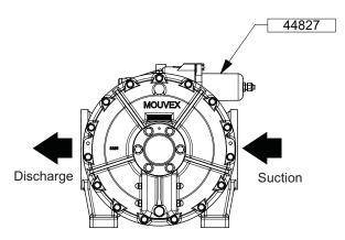
This control is not necessary in the case of a double internal relief valve, protecting the pump in both directions of operation.
