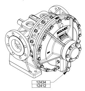
Once the pump is drained, fit the plug 12434 and its seal 12412.
