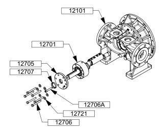
If necessary, fit the lip seal 12707, lip orientated outside in the bearing cover 12705.
