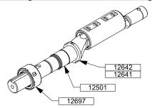
Remove the rotating part 12697 (the mechanical seal driver 12641 and its screws 12642) from shaft 12501 taking care not to scratch it.
