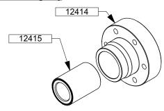
Orientate bushing chamfer on the outer side (see scheme above).
