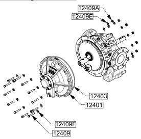
Remove the front cover bolts (screw 12409, nuts 12409A and washers 12409E - 12409F).
