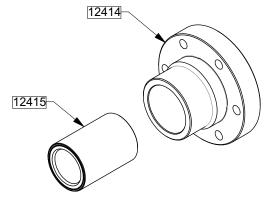
Orientate bushing chamfer on the outer side (see scheme above).
