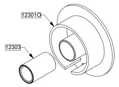
Remove the bushing 12303 of the piston 123010 with a press and a cylinder.
