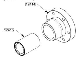
Remove the bushing 12415 of front cover bearing 12414 with a puller.
