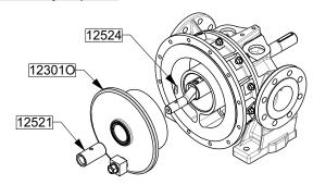
Lubricate the friction surfaces of the piston 12301O with a product compatible with the pumped liquid.
