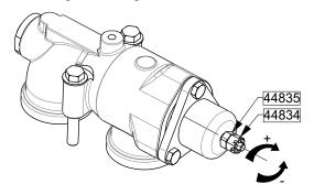
Setting is correct when flow rate is conform to expectation and when motor endures without incident absorbed power peak when discharge is closed. This is how relief valves of complete pumping sets are set, basing on information given to our technical services.
