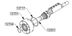
Remove the seal 12717 and check its condition. Replace it if necessary.
