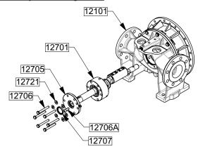
If necessary, fit the lip seal 12707, lip orientated outside in the bearing cover 12705.
