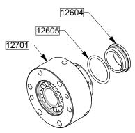
Remove the stationary seal face 12604 and its seal 12605
