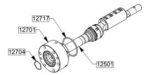
Fit the set bearing cage (12701 - 12703 - 12733 - 12627 and mechanical seal stationary seal face) on the shaft 12501.
