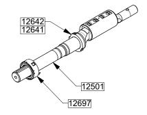
Check shaft 12501 surface condition. Rub it down with thin sand paper if there are scratches on seal rotating part O-ring place. In particular, it must be check that there are no scratches parallel to shaft axis.
