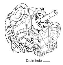
Fit the screws 12706 and theirs new ridged conic washers 12721 with medium thread lock.
