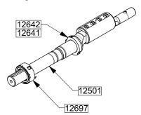
Remove the rotating part 12697 (the mechanical seal driver 12641 and its screws 12642) from shaft 12501 taking care not to scratch it.
