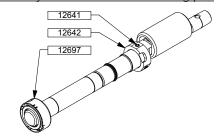
Check shaft 12501 surface condition. Rub it down with thin sand paper if there are scratches on seal rotating part O-ring place. In particular, it must be check that there are no scratches parallel to shaft axis.
