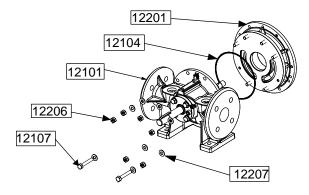
Remove the nuts 12206, the screws 12107 and theirs washers 12207.
