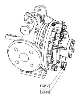
Once the pump is drained, fit the plug 12434 and its seal 12412.
