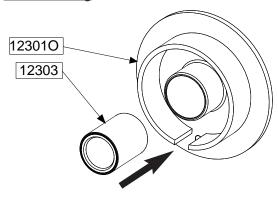
Insert the bushing 12303 in the piston 123010 with a press and a cylinder until the faces of the bushing and the piston are aligned (on both sides).
