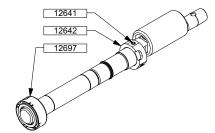
Remove the rotating part 12697 (the mechanical seal driver 12641 and its screws 12642) from shaft 12501 taking care not to scratch it.
