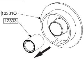
Remove the bushing 12303 of the piston 123010 with a press and a cylinder.
