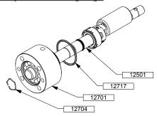
Fit the set bearing cage (12701 - 12703 - 12731 - 12733 - 12627 and mechanical seal stationary seal face) on the shaft 12501.
