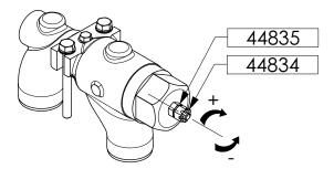
Setting is correct when flow rate is conform to expectation and when motor endures without incident absorbed power peak when discharge is closed. This is how relief valves of complete pumping sets are set, basing on information given to our technical services.
