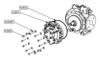
Remove the front cover screws (screw 12409, 12409D and 12409G and washers 12409F).
