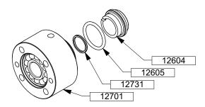
Remove the stationary seal face 12604 and its seal 12605.
