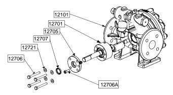
If necessary, fit the lip seal 12707, lip orientated outside in the bearing cover 12705.
