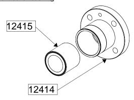
Orientate bushing chamfer on the outer side.
