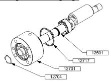
Remove the seal 12717 and check its condition. Replace it if necessary.
