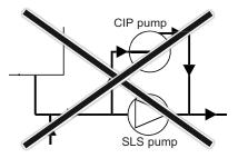
Indeed, in this case, the pressure at the inlet of the SLS Series pump is lower than the pressure at the discharge and the piston remains forced against the cylinder. Therefore, there the SLS Series pump no longer provides a passage. Its efficient cleaning can no longer be ensured and the cylinder/piston pair will become prematurely worn.
