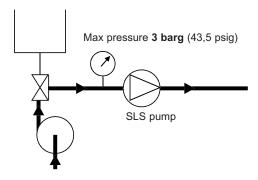
It is preferable not to run the SLS Series pump during CIP although low speed (< 100 rpm) is acceptable by alternating start/stop operation.
