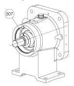
Re-mount the cover 607 after placing the seal 602, greasing the lips of the seals and greasing between the 2 seals 608.
