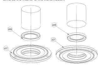
If the seal face is marked, change the ring 507. Break the ring with a chisel then fit a new ring after heating it at 90°C (in an oil bath or at HF).
