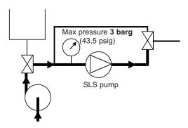
It is preferable not to run the SLS Series pump during CIP although low speed (< 100 rpm) is acceptable by alternating start/stop operation.
