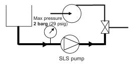
We recommend limiting the rotation speed of the SLS Series pump.
