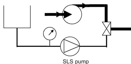
The SL Series pump is stopped when cleaning the installation.
