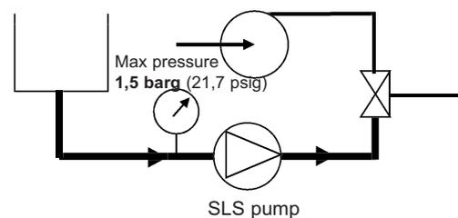
We recommend limiting the rotation speed of the SL Series pump.
