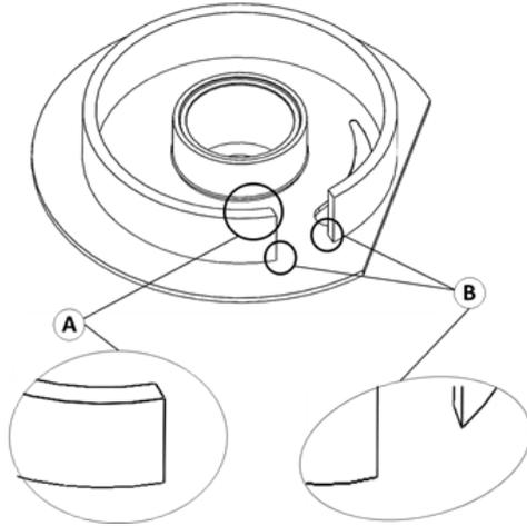
**Do not retouch any other surface of the piston by any mean as it can degrade pump performance and reliability. In particular, do not round or attenuate disc wall edges.**
