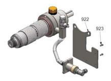
• On the spare transmission, remove the 2 screws 921 and the two screws 923 and remove the transport / storage bracket 922B.
