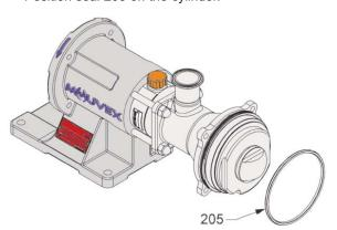
Re-mount front cover 400 while positioning the outlet port as desired.
