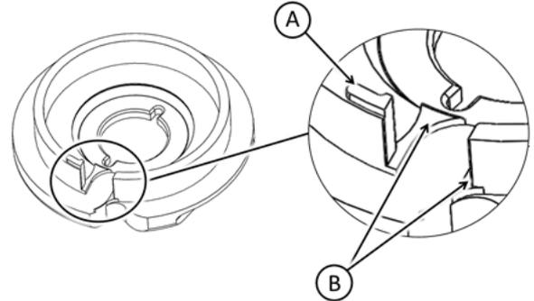
Before putting back the piston on the pump, eliminate these asperities by filing and finishing with fine sandpaper (No 320 grain or equivalent), taking care of not scratching any other surface around. Piston must then look as follows :
