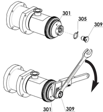
**Pumps manufactured after September 2014** : Groove under transmission hub.
