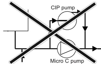
Indeed, in this case, the pressure at the inlet of the Micro C pump is lower than the pressure at the discharge and the piston remains forced against the cylinder. Therefore, the Micro C pump no longer provides a passage. Its efficient cleaning can no longer be ensured and the cylinder/piston pair will become prematurely worn.
