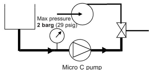
We recommend limiting the rotation speed of the Micro C pump.
