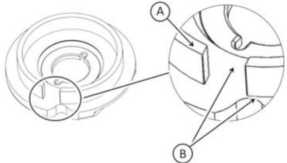
**Do not retouch any other surface of the piston by any mean as it can degrade pump performance and reliability. In particular, do not round or attenuate disc wall edges.**
