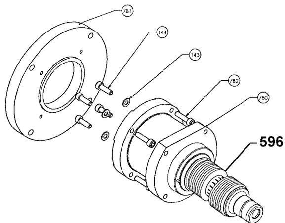
The trunk is dismantled by dismantling the front cover and manifold as explained in the DISASSEMBLY paragraph.
