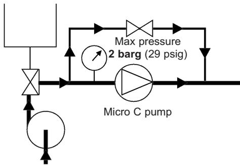
It is preferable not to run the Micro C pump during CIP although low speed (< 100 rpm) is acceptable by alternating start/stop operation.
