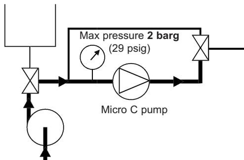
It is preferable not to run the Micro C pump during CIP although low speed (< 100 rpm) is acceptable by alternating start/stop operation.
