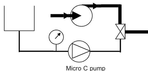
The Micro C pump is stopped when cleaning the installation.
