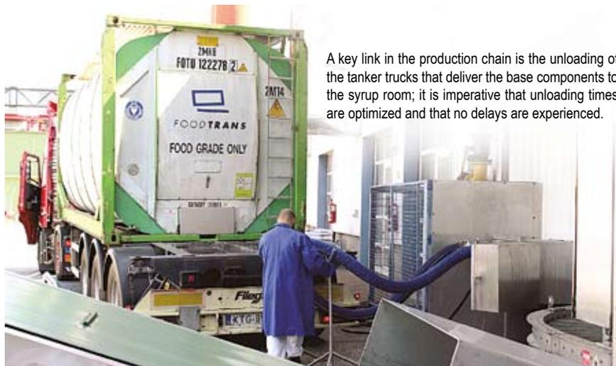
A key link in the production chain is the unloading of the tanker trucks that deliver the base components to the syrup room; it is imperative that unloading times are optimized and that no delays are experienced.
