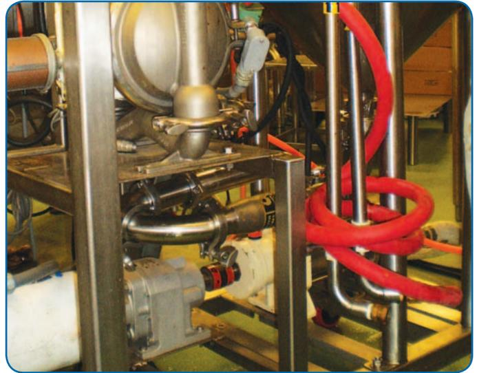
The Mouvex C-Series pump is easy to maintain and can be cleaned in place (CIP).
