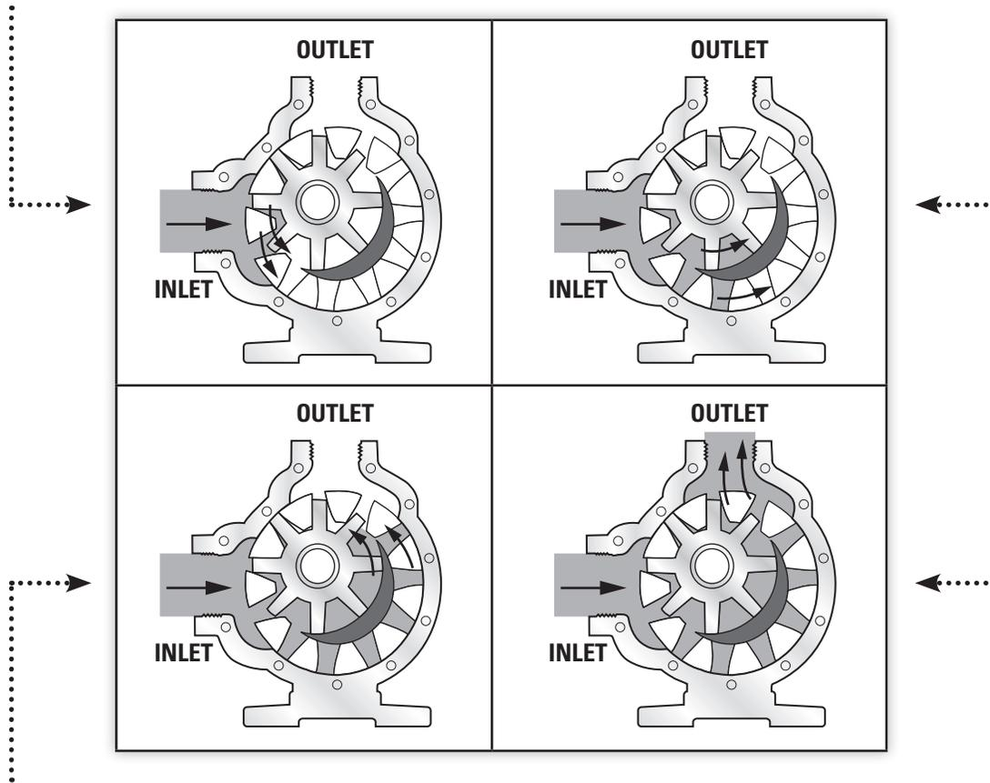
**3** As the rotor continues to turn, the liquid is forced past the crescent-shaped area and moves toward the discharge port.
