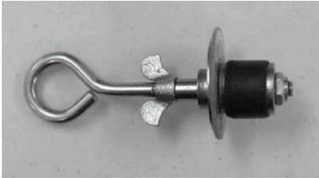
Pump Disassembly Tool F-00097
