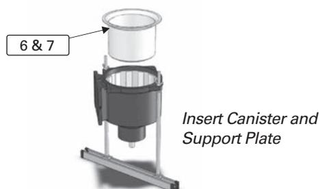
*Insert Canister and Support Plate*
