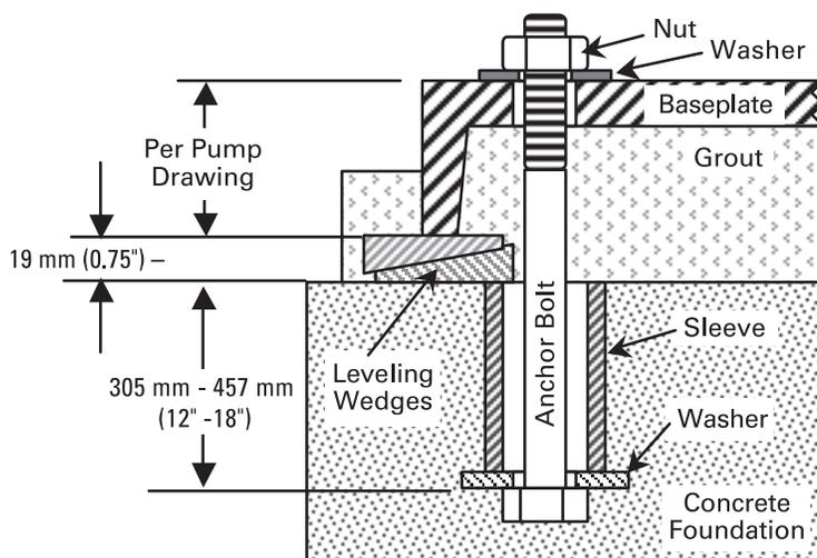
TYPICAL ANCHOR BOLT (SLEEVE TYPE)
