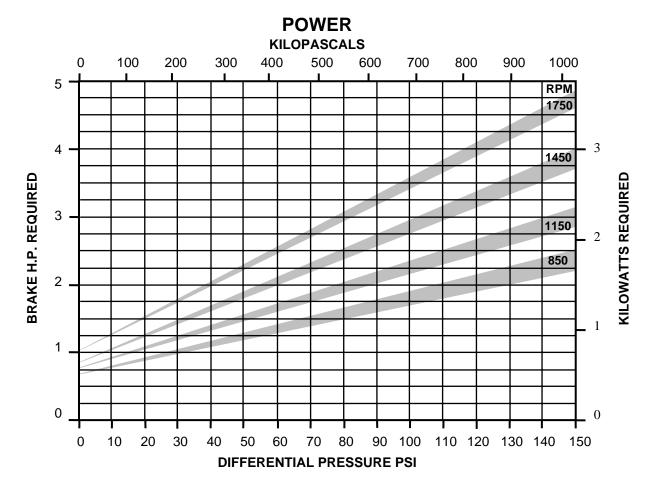
**NOTE:** Blackmer Characteristic curves are based on Brake Horsepower (BHP). To determine Motor Horsepower, drive train inefficiencies must be added to the BHP.
