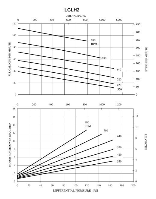
Blackmer Characteristic Curves are based on Brake Horsepower (BHp). To determine Motor Horsepower, drive train inefficiencies must be added to the BHp.
