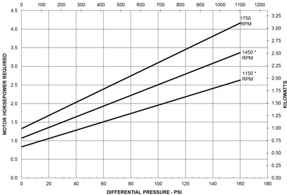
\*1150 and 1450 RPM curves are estimations based on 1750 RPM testing.
