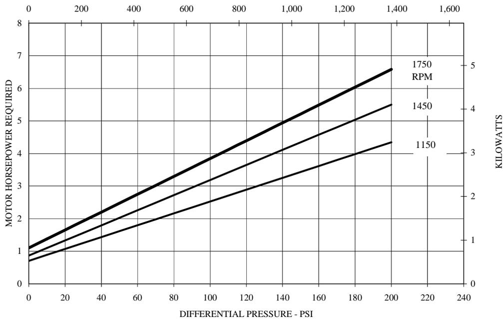
Blackmer Characteristic Curves are based on Brake Horsepower (BHp). To determine Motor Horsepower, drive train inefficiencies must be added to the BHp.
