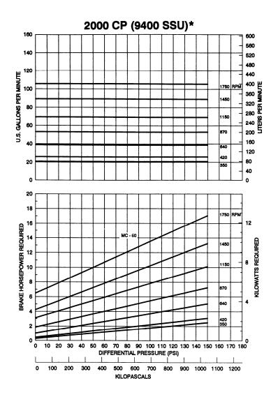
**NOTE:** The MC (dotted) lines are provided to assist in magnetic coupling selection. The MC lines can be used for operating temperatures up to 200°F (93°C). For higher temperatures, consult factory.
