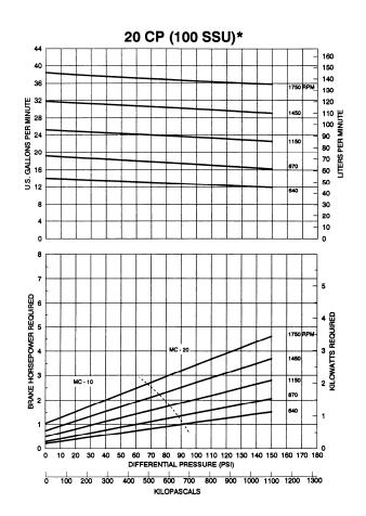
**NOTE:** The MC (dotted) lines are provided to assist in magnetic coupling selection. The MC lines can be used for operating temperatures up to 200°F (93°C). For higher temperatures, consult factory. For viscosities greater than 1000 CP (4600 SSU), consult factory.
