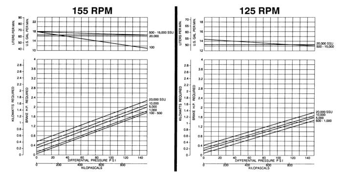
**NOTE:** Blackmer Characteristic Curves are based on Brake Horsepower (bhp). To determine Motor Horsepower, drive train inefficiencies must be added to the bhp.
