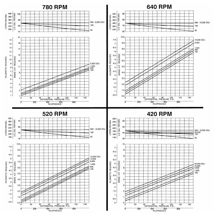
**NOTE:** Blackmer Characteristic Curves are based on Brake Horsepower (bhp). To determine Motor Horsepower, drive train inefficiencies must be added to the bhp.
