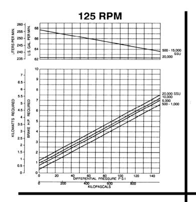
**NOTE:** Blackmer Characteristic Curves are based on Brake Horsepower (bhp). To determine Motor Horsepower, drive train inefficiencies must be added to the bhp.
